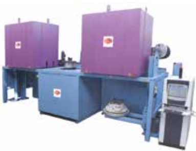
Additional quench furnace fully equipped
